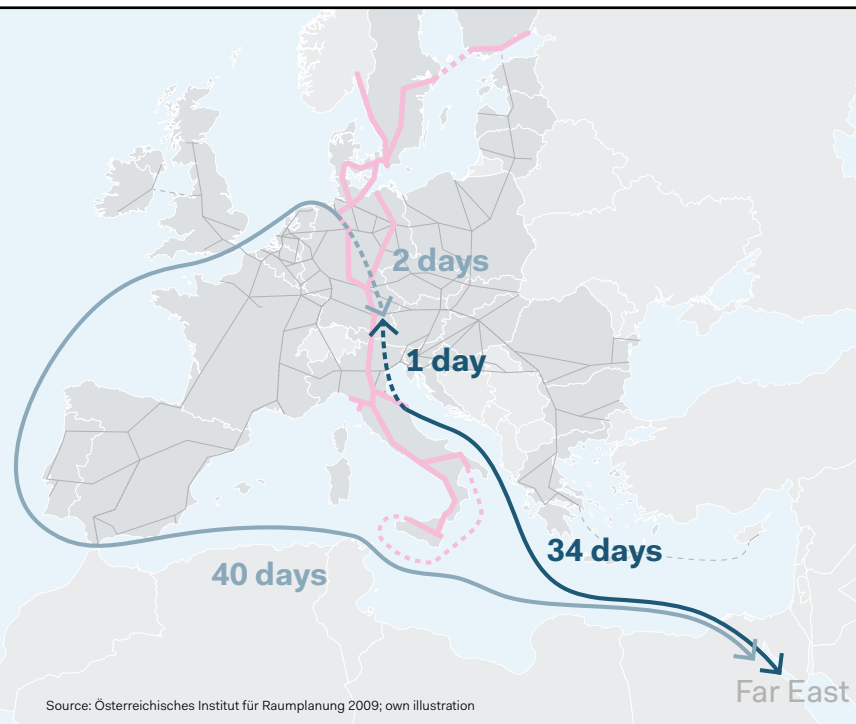
Comparison of transport times between the Far East and South Germany via Adria and North Sea ports
